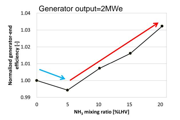
Generator-end efficiency,  $\eta_{GE}$  $\eta_{GE} = 100 \times \frac{Generator \ output}{Total \ fuel \ energy \ input}$
