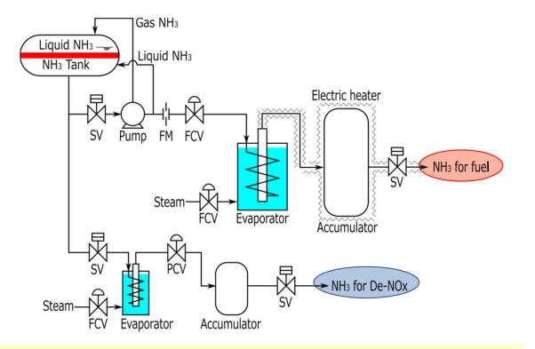
• Liquid NH<sub>3</sub> pressurized by canned motor pump and
