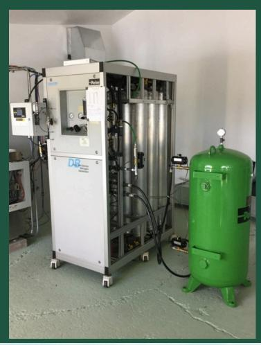
The Ammonia Shed is a 10 x 10 foot building that contains the inlet and outlet cylinders, the Reactor, and all the valves and pumps to produce NH3 stored in the mini nurse tank.
