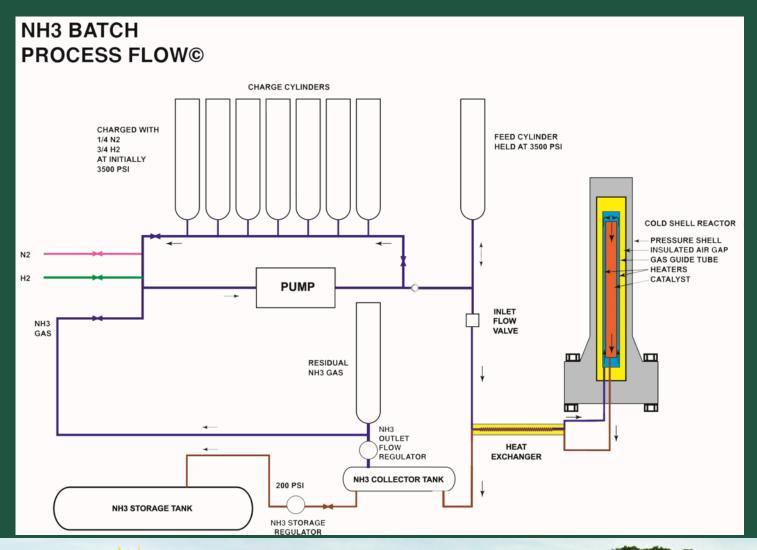
The gases flow from the blue cylinders through the reactor to the red cylinder converting 3500 psi nitrogen and hydrogen gases to ammonia at a rate of 6.72 lbs/hour, or 1.31 gallons/hour.
