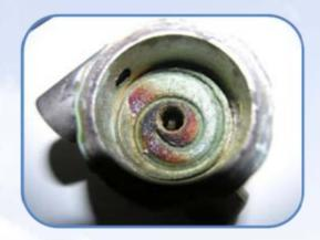
Concerning the **ammonia injector**, the rubbing of the mobile magnet on its guide led to a partial removal of the original coating **exposing metal to gaseous ammonia**.
