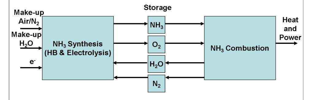
Very difficult for a combustion engine to double as a compressor/ chemical reactor! Result: not a unified device.
