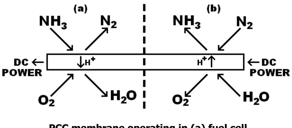
PCC membrane operating in (a) fuel cell and (b) fuel synthesis modes.
