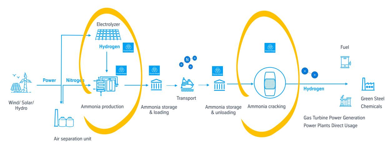
Ammonia usage for energy transport, utilization as energy carrier or re-conversion to hydrogen
