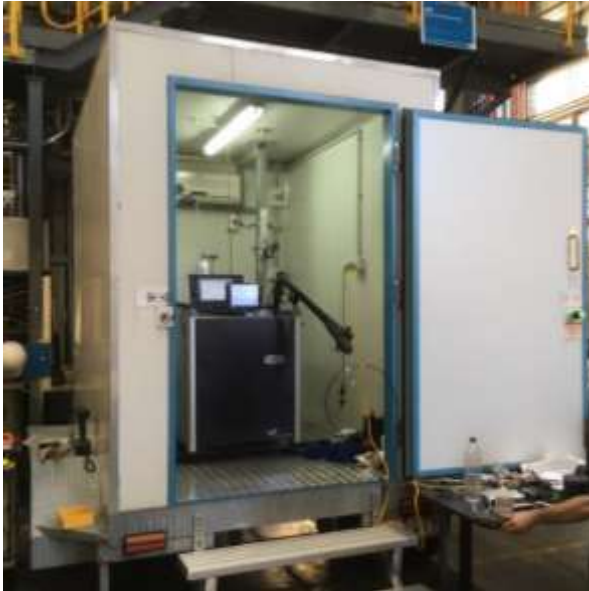
Trailer-mounted SYFT Voice 200 Secondary Ion Flow Tube Mass Spectrometer (SIFT-MS)
